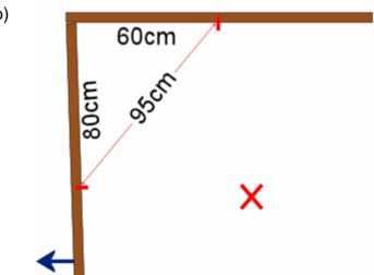
To make the corner square in this instance it would be necessary to move the wall frame outwards until the correct distance of 100cm could be obtained.
