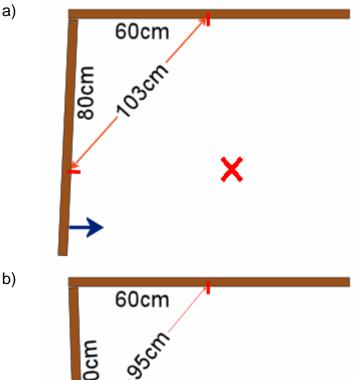
To make a right angle (or square corner in construction) it would be necessary to close the gap by moving the wall frame inwards until the length between marks was 100cm.
