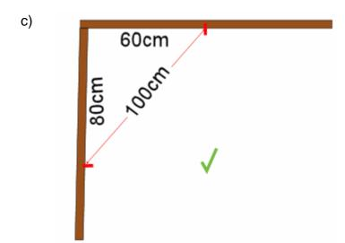
In this case, the two wall frames would be perpendicular to each other.
